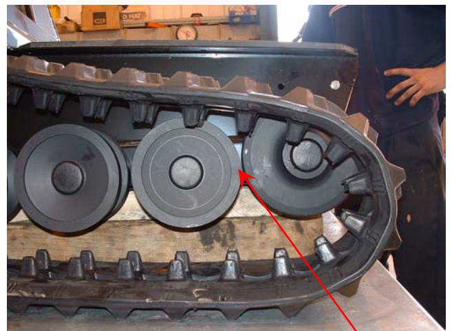
Adjust until idler is in line with roller
