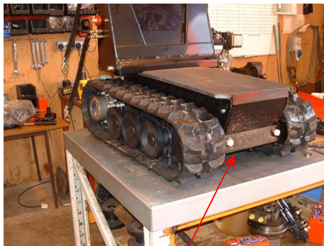
Remove any blocking under chassis run and test.
