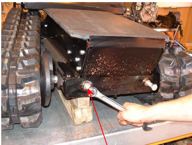
Insert jacking bolts adjust equally
