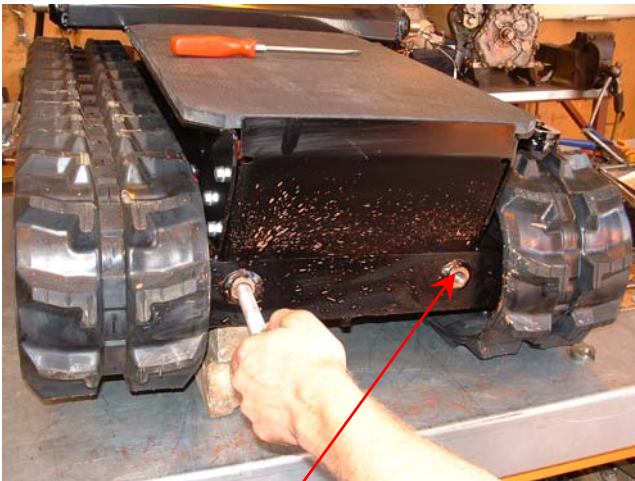
Remove jacking bolts
