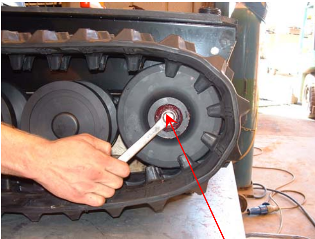
Install securing bolt (torque 49Nm)
