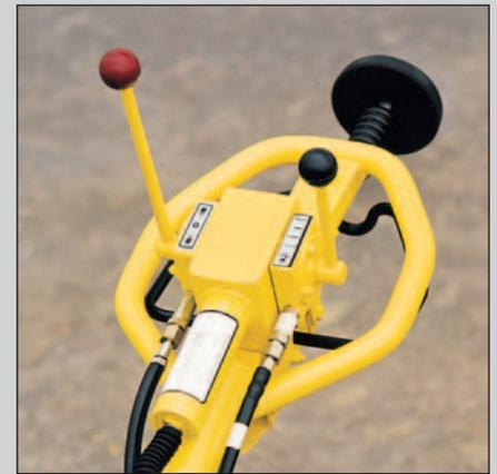
Steering arm with reversing protection and safety shut-down, CE conformity.
