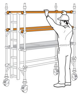
**3** Fit two diagonal braces in opposing directions between the 1<sup>st</sup> and 3<sup>rd</sup> rungs. Ensure that the frames are vertical and level by checking with a spirit level and setting the adjustable legs as necessary. Fit stabilisers (see notes on **page 9**). Fit the next pair of end frames and check the frame interlock clips are engaged.
