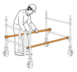
Fit two additional end frames, ensuring the frame interlock clips are engaged. Fit two diagonal braces (blue) in opposing directions, between the 1<sup>st</sup> and the 3<sup>rd</sup> rungs. Ensure the frames are vertical and level by checking with a spirit level and setting the adjustable legs as required.
