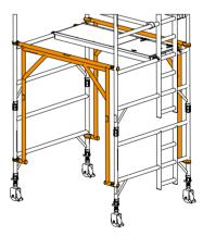
If end walk-through access is required at the base of 2.2m, 4.2m, 6.2m, 8.2m, 10.2m or 12.2m platform height, 1450 wide towers, walk-through frames may be used.
