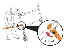
**3** Position the ladder frame as shown and fit the other end of the horizontal brace on to the vertical (just above the bottom rung). Fit a second horizontal brace between the bottom rungs on the other side of the frames to square the tower.
