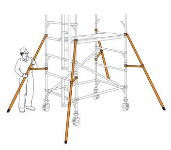
**6** Fit the next pair of diagonal braces in opposing directions between the 3<sup>rd</sup> and 5<sup>th</sup> rungs. Add two additional end frames.
